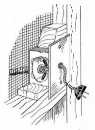
Fig. 2. Method of connecting Tobe Filterette to Diathermy screen.
