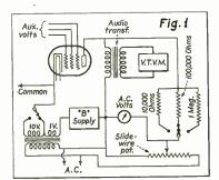
Schematic diagram of the plateimpedance bridge.
