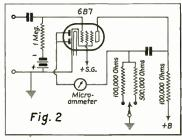
Schematic diagram of the vacuum-tube voltmeter.
