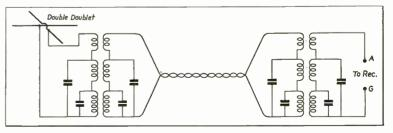
Fig. 2. Circuit of high-efficiency all-wave antenna system.
