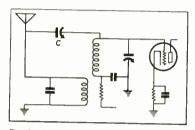
Fig. 3. Circuit of antenna coupling system.
