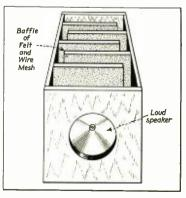
Fig. 9. Speaker with acoustic labyrinth composed of felt pads.
