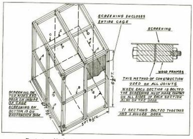
Fig. 1. Assembly drawing showing construction of Diathermy screen.
