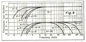
Two families of transmission loss—frequency ratio curves plotted from equation 7.
