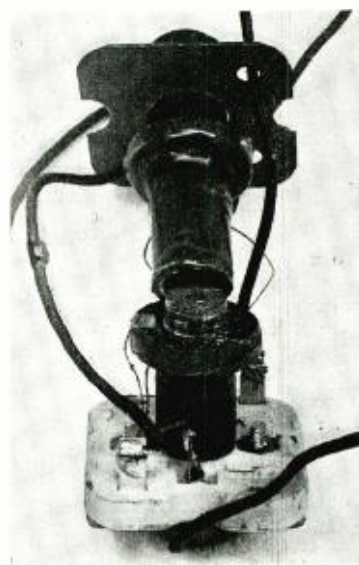
Fig. 2. Intermediate-frequency transformer broken open to show the character and position of one of the iron plug cores. A similar core is inside the upper part of the tubing. The coils may be wound directly on the plug cores, if desired.
