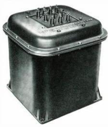
The output transformer illustrated, designed either for 204A's or 849's in class B, has a linear response from 30 to 12,000 cycles. The unit is oil immersed and shielded in a heavy gauge high permeability casting. All leads are terminated in high tension ceramic bushings. The transformer is insulated for 20,000 volts and will handle 1,000 watts audio power.
