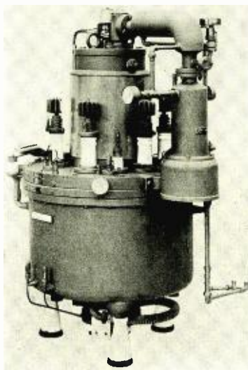
The new grid-controlled steel rectifier tube. Vacuum is maintained with a pump.
