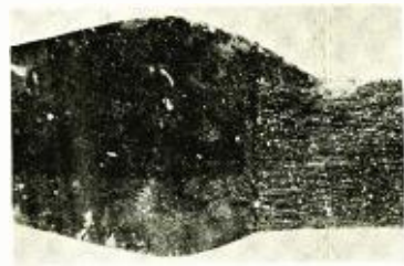
Fig. 5. Tungsten rod to copper strand; no sleeve. Showing the weakness of the weld. 50 x.
