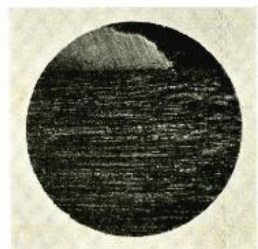
Fig. 4. Enlarged view of above showing no crystallization of tungsten when composite strand is used. 200 x.
