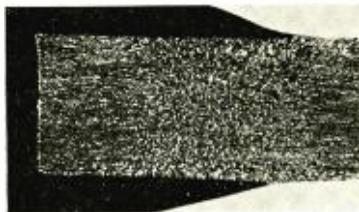
Fig. 1. Tungsten rod to stranded copper with nickel sleeve. 50 x.
