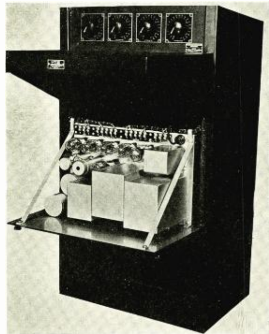
Fig. 2. The mounted amplifier tilted forward to show accessibility.
