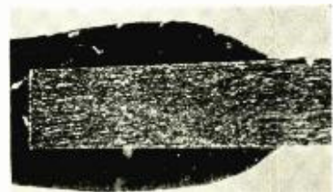
Fig. 6. Tungsten rod to composite strand; no sleeve. This shows the strong, well-balanced weld when composite strand is used. 50 x.
