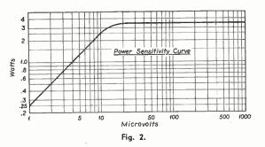
point where it is satisfactory, commercially. Many problems had to be overcome. Chiefly they were the ones of proper contact-point design and the elimination of sparking at the points. Unless properly designed, vibrator type power supplies creat intense r-f. disturbances which are picked up by the receiver making satisfactory reception impossible. The efficiency of a good unit runs quite high, perhaps 65 per cent.
