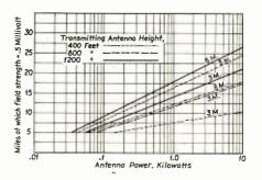
Fig. 4. Half-millivolt range versus kilowatts.
