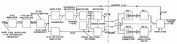
Schematic diagram of Western Electric equipment for common frequency broadcasting.
