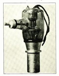
Fig. 6. Type 846 ultra-short wave tube. Normal power output: 1,000 w.
