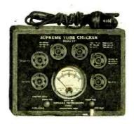
graved on the panel. There are no rheostats to regulate. Tests both types of type -80 rectifier tubes separately. It has a standard milliammeter, genuine D'Arsonval movement (either Jewel) or Weston meter). It is housed in a moulded bakelite case with carry-
