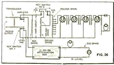
Illustrating function of key switch in relation to resistance network.
