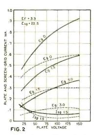
Plate and screen-grid current, at 22½ volts.
