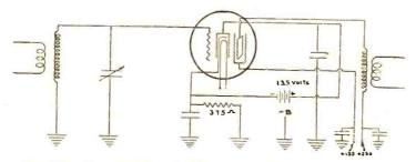
Connections of a-c. pentode used with separate battery for space charge grid
