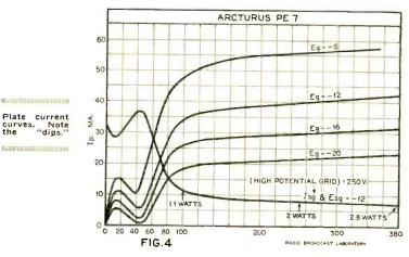
grid located between the control grid and the plate may not only reduce the space charge somewhat (Fig. 2) and make possible a tube with an amplification factor of 400 with a resistance of only 400,000 ohms but at the same time the extra grid at a high d-c. potential but low r-f. potential relative to the filament, effectively shields the control grid from the plate. In other words, it reduces the grid-plate capacity in the manner described many times in popular and technical literature.
