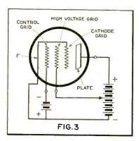
It is possible for a single electron to knock as many as twenty of its companions loose from the plate. If the total number which leaves the plate by this manner is equal to the number that stay there from the filament, the actual plate current is zero. If the number leaving is greater than the number arriving the plate current goes backwards. See Fig. 2.
