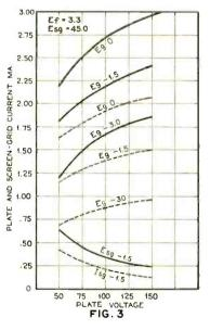
Plate and screen-grld current at 45 volts.
