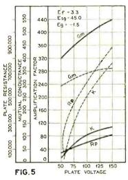
Amplification constant, plate resistance and mutual conductance at various plate voltages.
