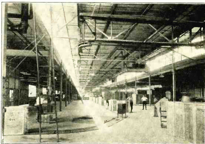
Here is the Crosley Radio Corporation's shipping room, where, by means of a carousel conveyor, radio sets can be carried to waiting freight cars at the rate of 580 per hour.
