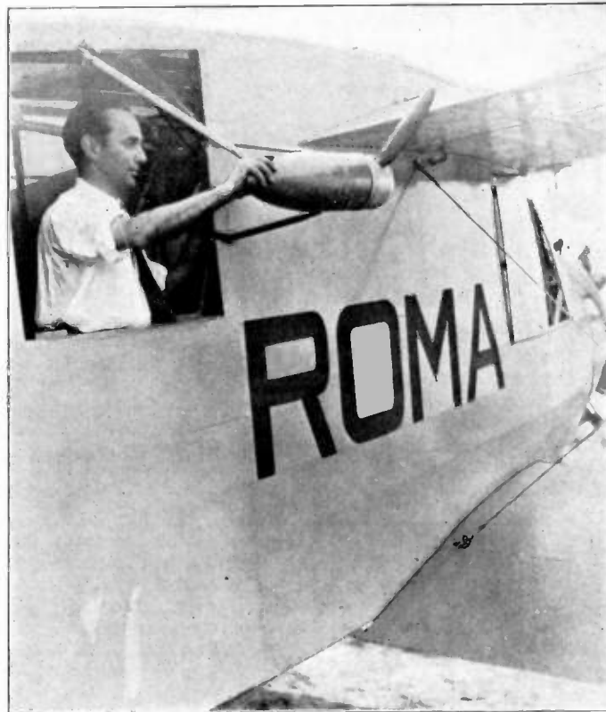
The wind-driven generator swung out of the cabin to operating position. This generator supplies both high and low voltages for operation of the transmitter. It may be drawn into the cabin when not in use thus reducing wind resistance.
