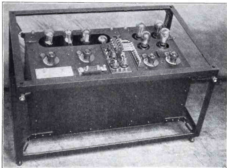
The transmitter and receiver of the simplex train communication equipment. The transmitting unit, which utilizes three 50-watt tubes, is on the left. Four 7½-watt tubes are used in the receiver.
