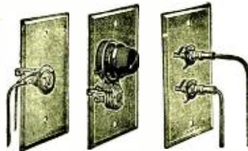
Special jacks and a combination jack and volume control designed for use in buildings wired for radio
