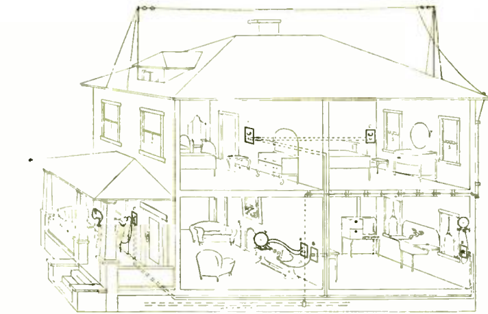
Fig. 1. Typical example of radio house wiring. A is an aerial and ground outlet jack; B, receptacle jack; and C, receptacle jack with volume control
