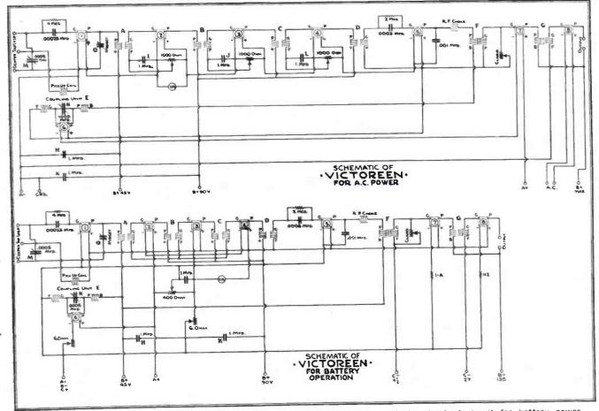
Circuit diagram of the Victoreen wired for operation from an ABC Eliminator, and the standard circuit for battery power Page 667 Radio Engineering, April, 1927
