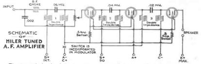
The general circuit of the tuned double impedance amplifier. Variations of this circuit are covered in the article
