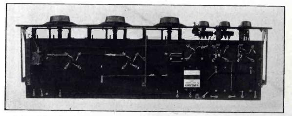
Underneath the sub-panel of the A. C. operated T.R.F. set. Note the fixed resistances, connected to the filament posts of the R.F. sockets, and which are used to provide a negative blas on the R.F. tubes
