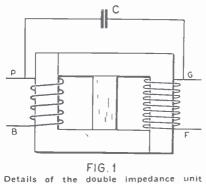
It provides complete magnetic shielding, so that radio frequency currents are eliminated from the audio circuits,
