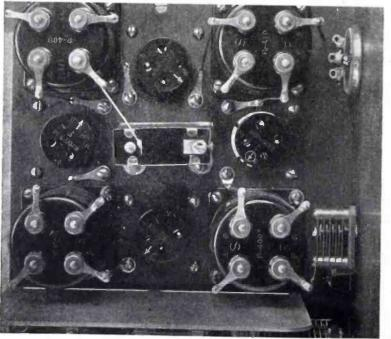
Details of the mounting and connections of the intermediate amplifier. Very short leads are used for all high potential wiring
