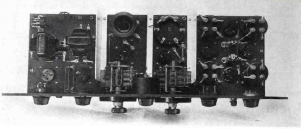
Bird's eye view of the Portable Super, completely wired and ready for Installation in its carrying case. Practically every available Inch of space is occupied by an efficient and compact grouping of apparatus
