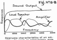
plifier to work in conjunction with a cone loudspeaker
