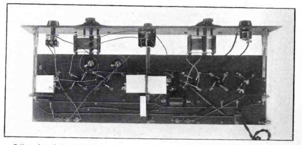
Bottom view of the new Victoreen. The potentic meters controlling the second and third intermediate tubes are mounted on the sub-panel, as shown. Flex ible connections are made between the front panel apparatus and the sub-panel units and, since the mounting brackets are adjustable, a sloping front cabinet can be used, if desired
