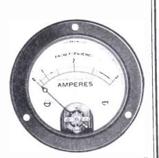
Pattern No. 135—Movement parts are all silvered and the scale is silver etched with black characters. The case diameter is two inches and can be furnished in any desired finish, standard being black enamel. It is equipped with zero adjuster. as are all Jewell moving coil instruments.
