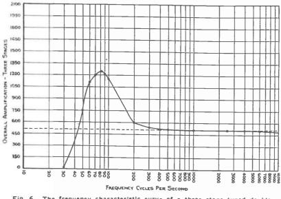
Fig. 6. The frequency characteristic curve of a three stage tuned double impedance amplifier. This will illustrate the rising characteristics of the amplifier at low frequencies
