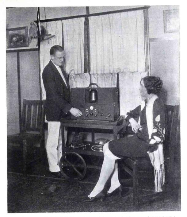
Complete set up of the Portable Super. The design of this receiver has been so worked out that it is adaptable to practically any installation requirements. Sufficient space is available in the cabinet for dry batteries, so that the outfit can moved easily.
