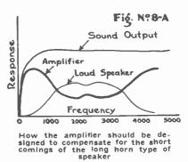
be chosen to exaggerate the low and with less response on the middle and still less on the high frequencies. Fig. 8b.
