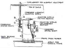
Fig. 3. Mechanism of the bearings and micrometer adjustment
