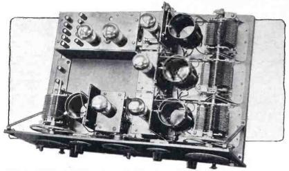
Fig. 1. The assembled receiver with the covers of the four tuning units removed.
