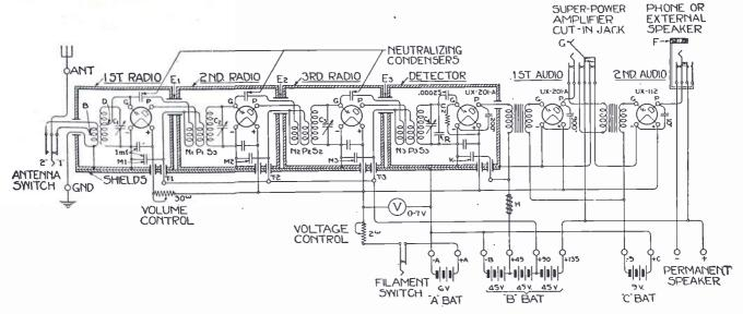
Fig. 5. All the circuit data on the Stromberg-Carison shielded neutrodyne is given in this diagram
