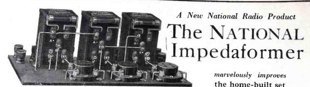
The Illustration Shows the Assembly of Three Impedaformers as They Would Appear in a Set
