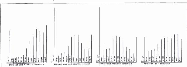
Fig. 2. The length of the vertical lines indicates the distance the dial must be turned to tune from one station to the next
