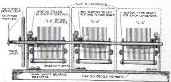
Fig. 2. Details of the triple condenser. Note that the three rotors are adjustably fastened to the solid steel shaft
