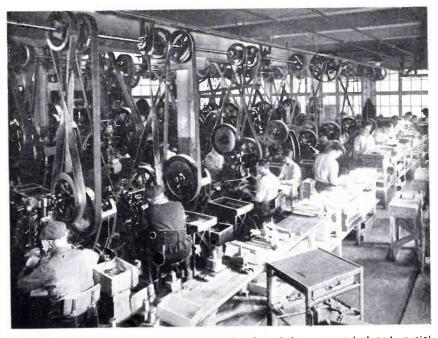
Fig. 2. A part of the stamping department, where holes are punched and special shapes stamped into the panels
