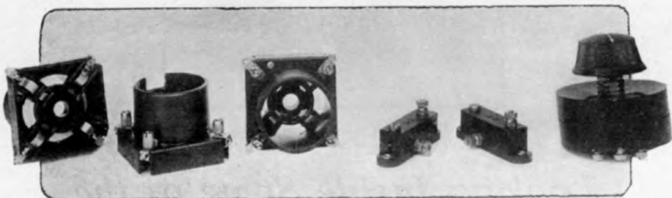
Fig. 1. Showing the new socket for UV or UX tubes, the neutralizing condenser, and special variable resistance.
