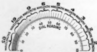
Ordinary Condenser Arrangement of Wavelengths Ordinary straight capacity condensers crowd 70 of the 100 wavelengths into the first 30 points of the dial.
