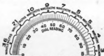
Straight Wavelength Condenser Arrangement With straight-line-wavelength condensers 57 of the 100 wavelengths are crowded into the first 30 points on the dial.
