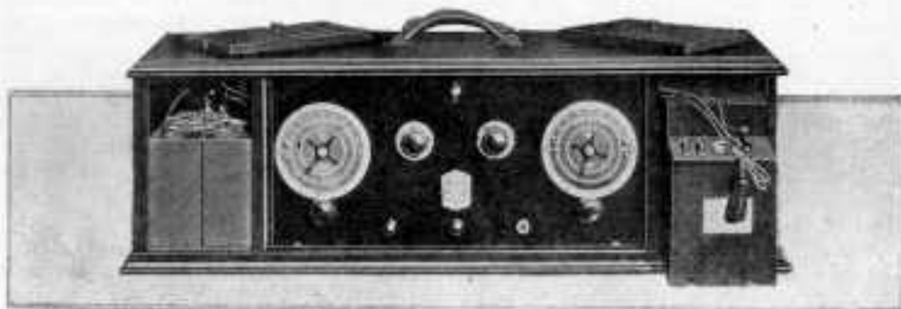
Fig. 5. Illustrating the method of installing the A type in a super-heterodyne. No special care for charging is required, as the battery floats on the line when the current is turned on at the electric light socket
