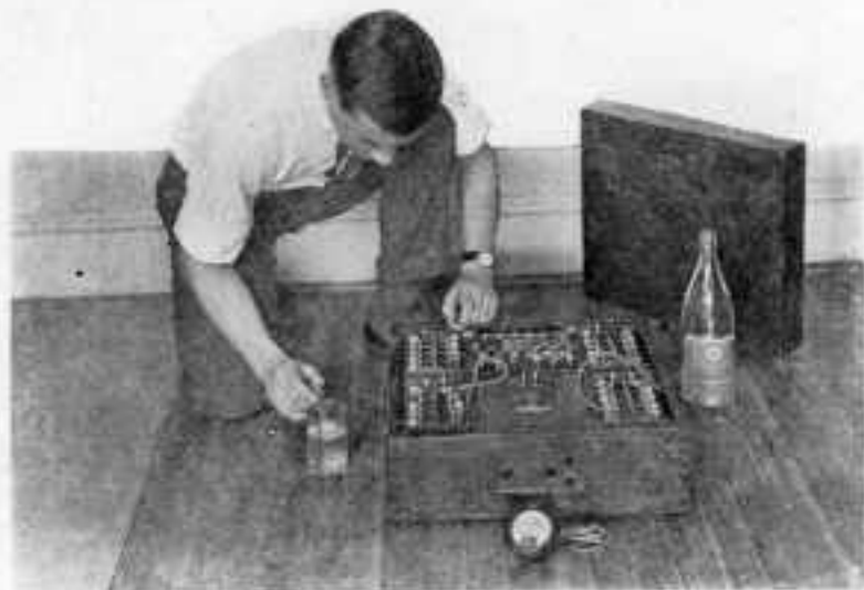
Fig. 2. It is no trouble to maintain the Unipower B, for only regular charging and periodic filling are all that is necessary. Use a high resistance voltmeter, such as the Weston or Jewel types, for measuring the voltage
