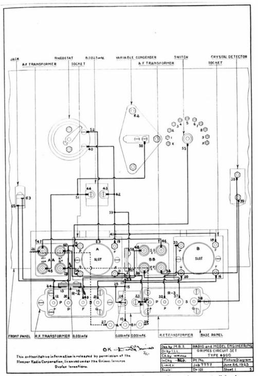
Fig. 8. Picture wiring diagram of the set, showing the connections as they are actually made
