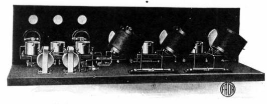
Showing the rear view of a five-tube Neutrodyne circuit radio receiver constructed according to information in the booklet "How to Build Hazeltine Neutrodyne Circuit Radio Receivers."
