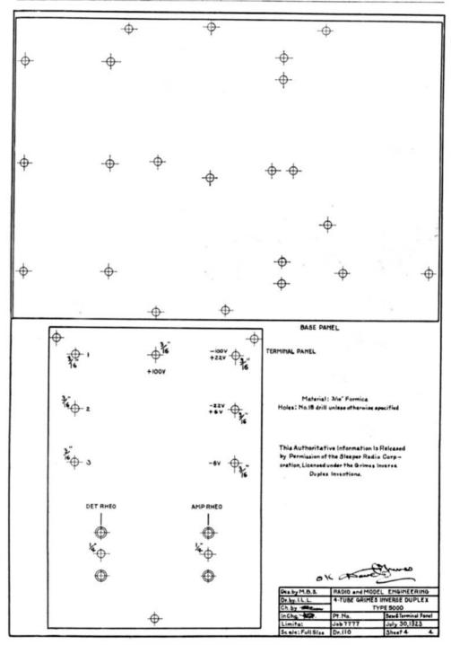
ig. 7. One-half scale drawing of the base and terminal panels. Engraving for the binding posts is also indicated
