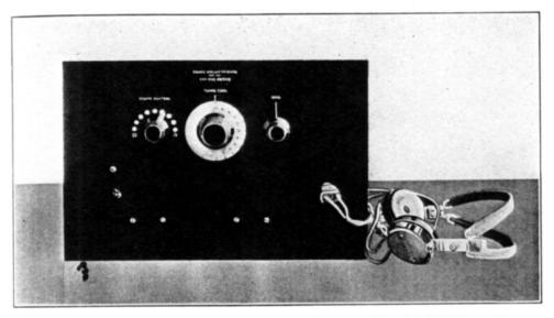
Fig. 1. The set ready to operate. Since the loop can be mounted directly behind the panel this makes a most convenient table unit
