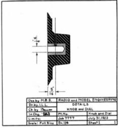
Fig. 6—The two important points of knob and dial design
