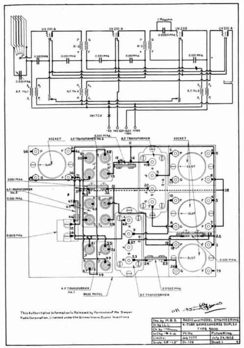
Fig. 8. Above is the schematic diagram, and below the picture wiring diagram of the base panel. No wires to the front or terminal panels are shown
