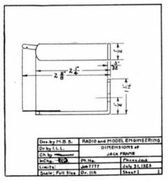
Fig. 8-Phone jack details at one-half scale
