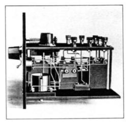
Fig. 5. Here the three audio transformers and the 0.005 mnd. condenser can be seen
