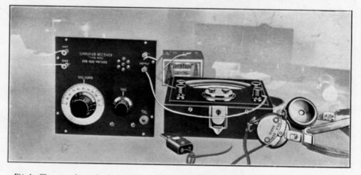
Fig. 1. The set as it was hooked up for measuring the plate current of the W. T. 501 tube. A Rawson micro-ammeter was used to indicate the current
