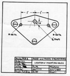
Fig. 3. Illustrating at one-half scale the standard arrangement of mounting screws
