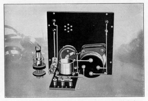
Fig. 2. A rear view of the Simplified Receiver, showing also the W. T. 501 tube mounted in the adapter
