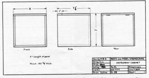
Fig. 2. The usual design for plain instrument cabinets, from which slight variations are sometimes made to give a slightly more ornamental appearance. Length X should be 7, 10, 14, 18 or 24 ins. according to the panel
