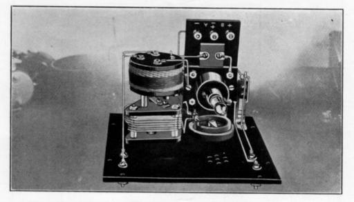
Fig. 3. Looking down on the set, with the tube in place. This shows clearly the tuning unit, as well as the other fittings
