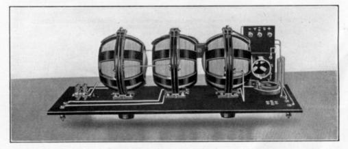
Fig. 3. The fact that so little wiring shows is due to the careful arrangement of the connections, rather than to the simplicity of the circuit
