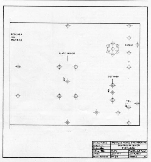
Fig. 6. The right hand half of the front panel, at one-half scale. Contentric circles indicate countersinking for flat head screws
