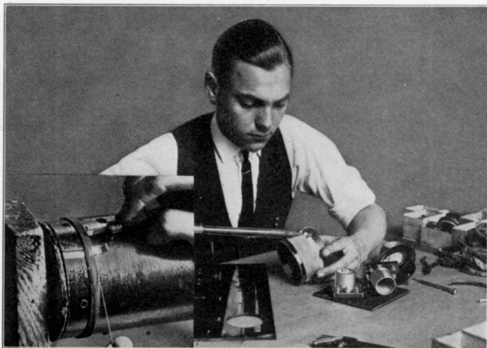
Fig. 1. Showing a new and very satisfactory method of tapping coils. Insert at left indicates position of copper strip.
