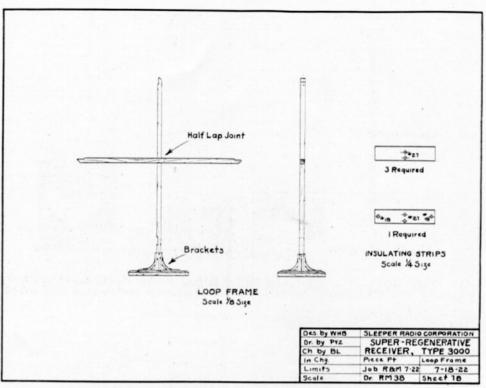
Fig. 7. A scale drawing of the loop frame and L. P. F. strips
