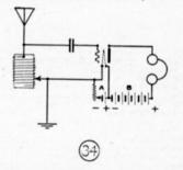
34. This is the simplest of audion detector receivers. A variable inductance is connected between the antenna and ground for tuning the outfit and the detector is wired to the same terminals. The grounded side of the tuner is connected to the filament while the antenna leads thru a fixed condenser to the grid. An A battery supplies the filament of the tube and a B battery in series with telephones maintains a positive charge on the plate.
