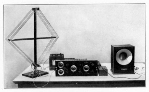
Fig. 8. Complete super-regenerative receiving equipment
