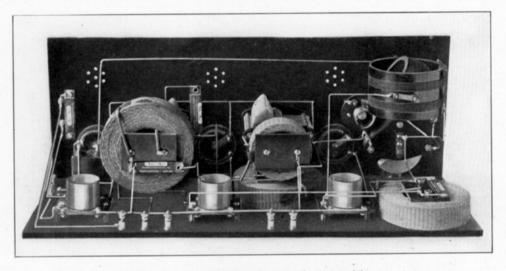
Fig. 3. Rear view which should assist in the wiring of the set
