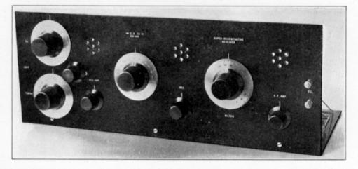
Fig. 1. A front view of the super-regenerative receiver
