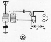
like charges being emitted from the filament and prevents a large number from reaching the plate. This reduces the current flowing thru the telephones. A positive charge on the grid has the opposite effect.
