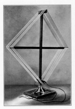
Fig. 6. The loop Antenna
