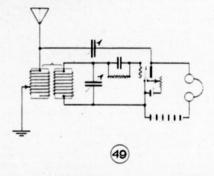
tion is almost identical with that of No. 42. 49. A simple method of obtaining regeneration is illustrated in this circuit. The system is essentially a loose coupler and audion detector with a variable condenser connected from the plate to the antenna. Tuning is accomplished in the usual way, while the coupling condenser is adjusted for the desired degree of feed-back. This method is more frequently employed for long wave reception than for short wave work.
