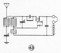
Where this result is obtained through the use of a separate oscillation generator the system is termed heterodyne, while autodyne is the name given to the method illustrated by this circuit.
