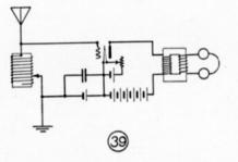
condenser is unnecessary. In this diagram a C battery of fixed value is shown, shunted by a condenser to by-pass radio frequency current.
