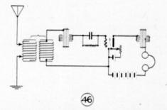
46. It will be noted that the chief difference between this circuit and the preceding one, is that a variometer instead of a variable condenser is used for tuning the grid circuit. It is a popular circuit among the advanced amateurs. The variocoupler stator is connected to the antenna and ground while the rotor is placed in series with the grid variometer and grid circuit of the detector. This comprises the tuning system, the plate variometer being used only to obtain regeneration.
