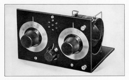
Fig. 1. Front view of the self modulated oscillator
