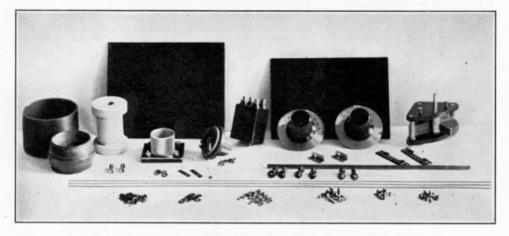
Fig. 5. Complete set of parts required for the construction of the oscillator
