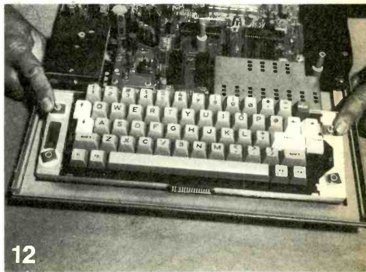
POSITION THE KEYBOARD over the plastic posts and let gravity do its work—gently. Secure the keyboard in place with the speednuts supplied with the kit.
