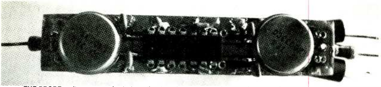
THE PROBE as it appears prior to insertion into the tubular casing. The input end is at the left. The IC's are shown in numerical order from left to right. The home-brew, printed-circuit board has foil surfaces top and bottom.
