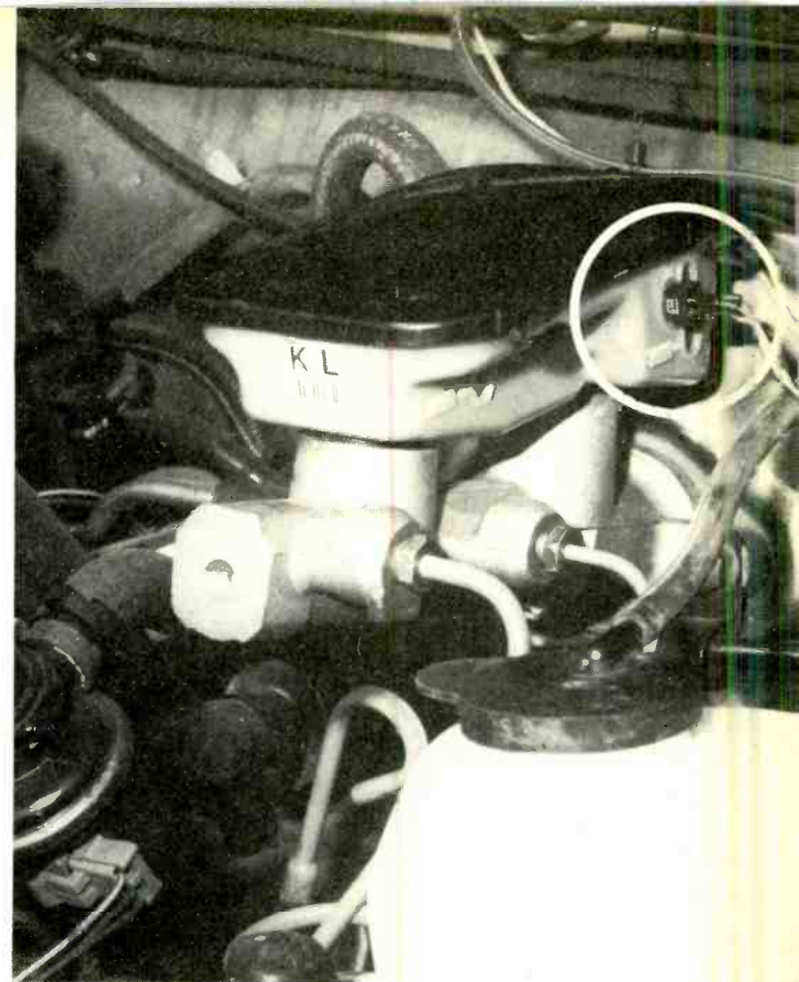
THE PLASTIC CONTAINERS for the master brake cylinder (center) and the window-washer fluid (lower right) were fitted with sensors (circle). Steering fluid container is not shown.
