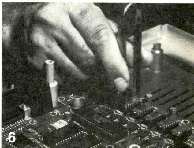
USE AN IC CHIP PULLER when removing the old IC chips to prevent accidental damage to the DIP sockets. Don't pry or flip the IC chips out with a screwdriver.
