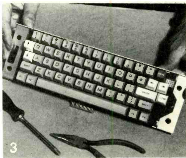
3 THE KEYBOARD is supplied as a complete factory-assembled unit that has been pretested. It is a direct substitute for the original Chiclet keyboard.
