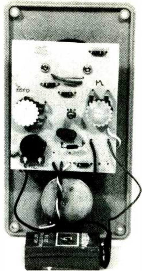
REAR VIEW OF THE FRONT PANEL shows printed-circuit board mounted on meter terminals—see two screwheads near top of board. Use a strip of double-sided tape to secure 9-volt battery to potentiometer case shown in lower part of photo.
