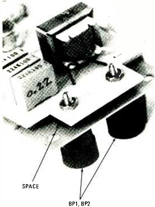
HERE'S A VIEW OF THE BOARD, SUPPORTED by the binding posts above the metal front panel of the plastic box. Check the space under the board as indicated in the photo and likewise under the screw mount at the other end. If wires and leads were cut close to the board, there should be no shorts at all.
