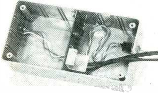
THE AC-POWERLINE WIRES PASS THROUGH A NOTCH cut into the end of the cabinet. They are secured when the cabinet cover is in place.
