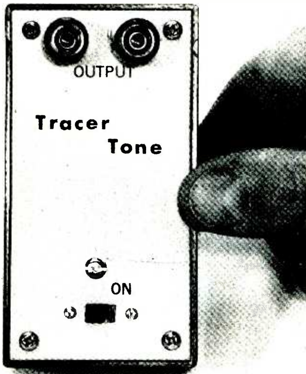
TRACER TONE ALL WIRED AND ASSEMBLED is ready for its first assignment with the toughest of wire harness or cable. If you wish, add an LED indicator and LED current-limiting resistor to the circuit so that you'll know when the switch is on. The intent is not to extend battery life, but to indicate to the wireman that the tone is being generated, and being pumped into the cable.
