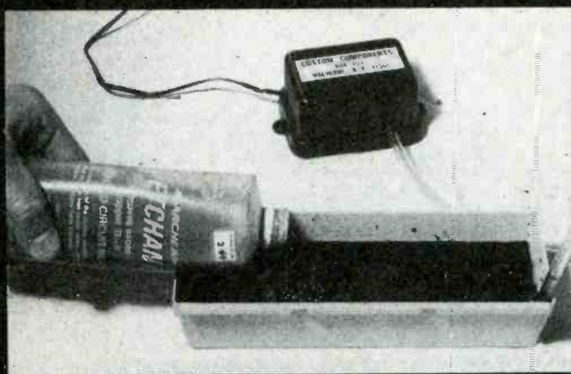
FIG. 7—TO ETCH A BOARD, fill the tray \frac{3}{4} full with etchant. Attach the air pump and power it up. Float the board on top of the etchant face down for the time period prescribed in the text.
