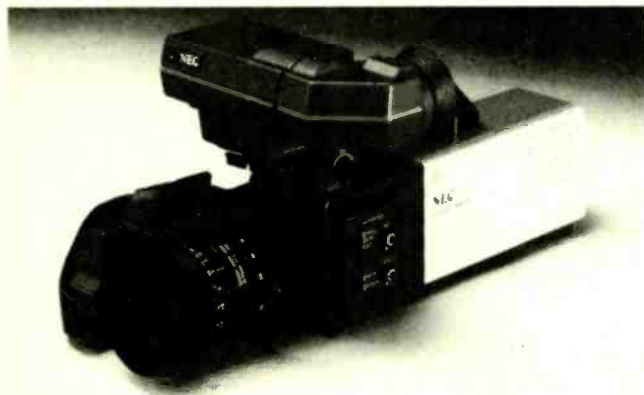
SOLID-STATE IMAGE SENSORS, such as the one used in this NEC TC-100 color camera may eventually replace the cumbersome and power-hungry image tubes of today.
