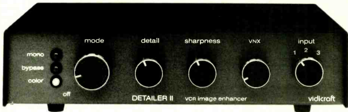
THE SHARPNESS AND DETAIL of both recorded and broadcast video can be improved by using an image enhancer.
