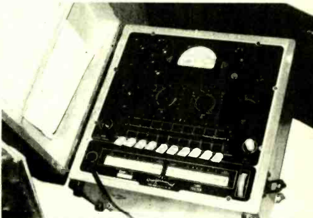
FIG. 4.—A TUBE TESTER can save you a lot of time and aggravation, especially if you buy a large numbers of used tubes.
