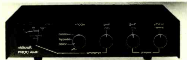
A TRUE PROCESSING AMPLIFIER, this unit from Vidicraft allows full control over both the color and sync of the video image.
