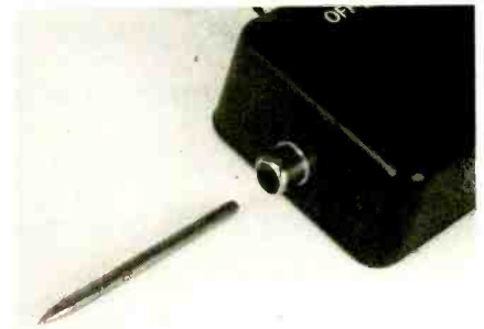
Fig. 4. A probe tip is easy to make by filing down a piece of 1/8-inch brass or steel rod. Rounding off the back end makes the probe needle easy to insert into J1. Not only does it fit securely into J1, it can be removed in order to make a direct cable connection to the Frequency Probe.
