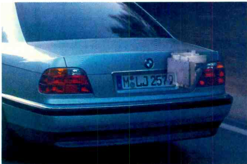
LOCATED IN THE TRUNK rather than under the hood, BMW envisions the fuel-cell as a replacement for today's lead-acid battery.
