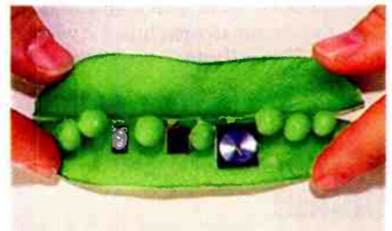
THE THREE MAIN COMPONENTS OF Sandia's micro-chem lab for gas-phase detection and analysis are small enough to fit easily inside a snowpea pod.
