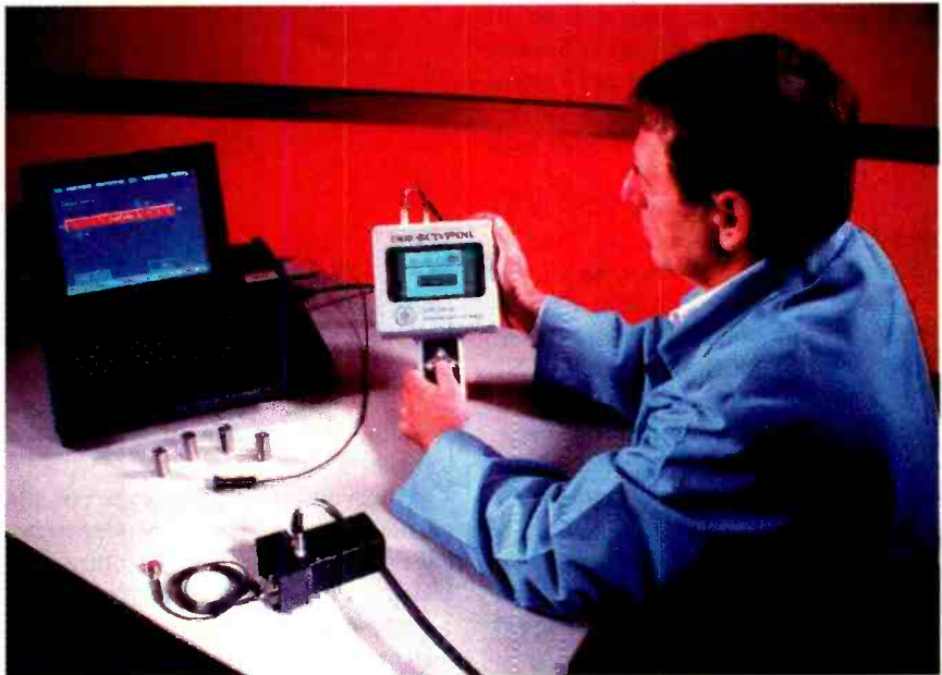
THE MATERIAL IDENTIFICATION SYSTEM is shown at the left attached to laptop computer. The engineer is holding the Ultrasonic Pulse Echo instrument.
