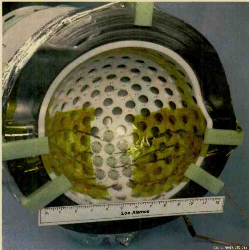
A CLOSE-UP VIEW OF THE WHOLE-HEAD MEG (magnetoencephalography) system "helmet". The white material is a newly patented material (DuPont/Los Alamos) that precisely holds each Superconducting Quantum Interference Device (SQUID) sensor in place.
