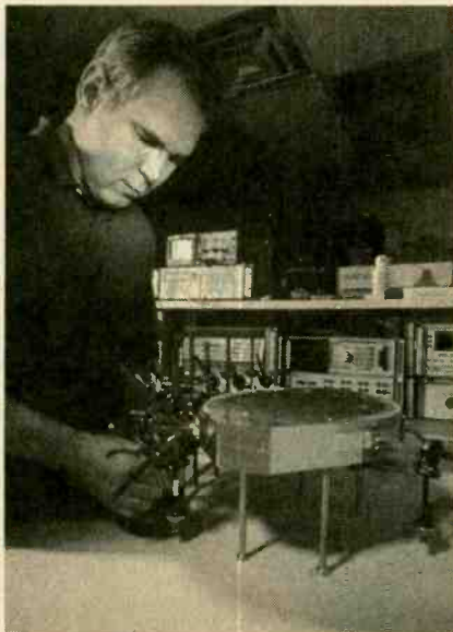
Here, Georgia Tech's Otto Rausch attaches waveguides to test his Rotman-lens antenna.
