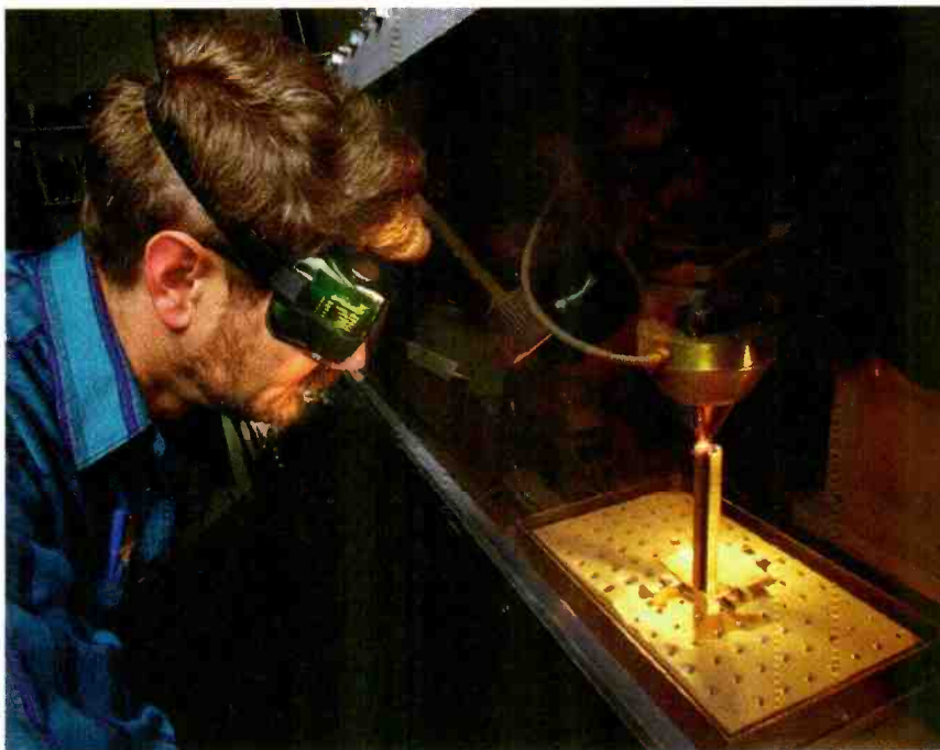
RESEARCHER LANE HARWELL MAKES AN 11-inch high mini skyscraper using Sandia's laser-engineered net-shaping technique.
