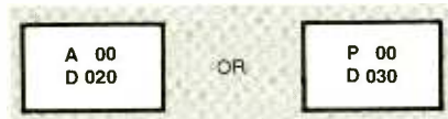
FIG. 3 —TO ENTER THE ADJUSTMENT system, use the right and left arrow keys to change the display from D000 to D030 in the Picture mode, and to D020 in the Audio mode.
