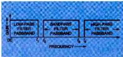
FIG. 1—IDEALIZED frequency-response curves for low-pass, bandpass and high-pass AC filter circuits.
