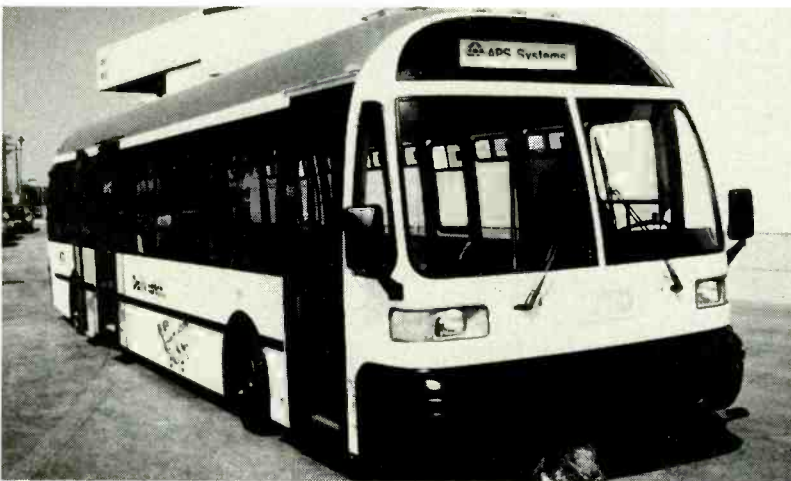
AN ELECTRIC BUS IN SANTA BARBARA, powered by nickel-cadmium batteries, will improve the air quality on downtown streets.
