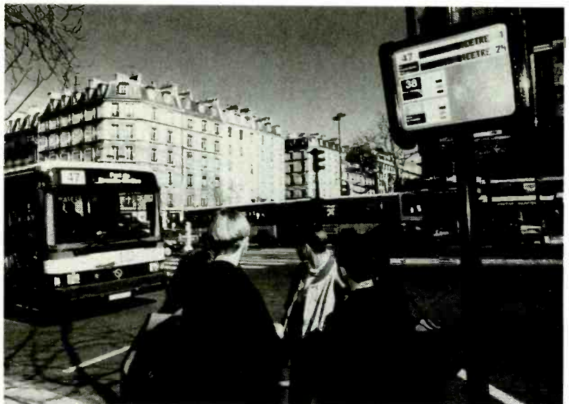
THE ALTAIR COMMUNICATION SYSTEM pinpoints bus locations in Paris with signals from GPS satellites. A liquid-crystal display at bus stops keep commuters informed of bus locations. Drivers and controllers can also keep tabs on bus locations and arrival times.
