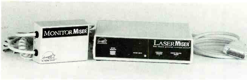
FIG. 5—MONITORMISER AND LASERMISER from EMPAC are companion energy savers that need no software to work. Both have DIP switches for setting their programming values. MonitorMiser uses a simple keyboard-sensing circuit to monitor PC activity. LaserMiser uses a microprocessor that analyzes and remembers your printing habits to power down a laser printer based on consumption.
