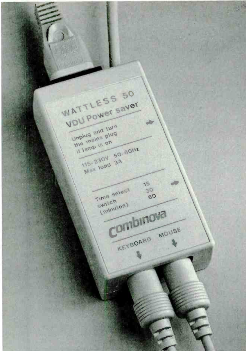
FIG. 4—TO INSTALL THE WATTLISS, unplug your keyboard, plug it into the Wattless, and then plug the Wattless keyboard cable into your PC. If you have a mouse, you can use a special cable with a bifurcated cord that allows you to plug it in as well.
