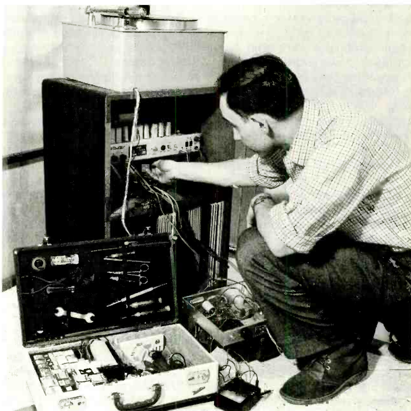
Young Larry Klein on a service call. Note the tubes and tools in the attache case service kit.
