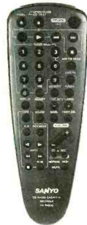
THE OUTPUT OF THIS remote control was "swamped" by an energy-efficient fluorescent tube.
