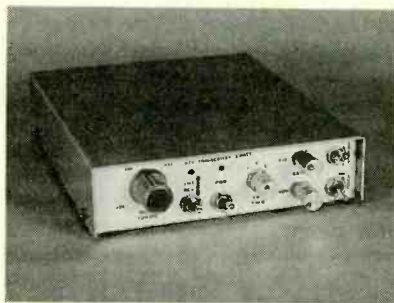
5-WATT ATV TRANSCEIVER. This small package contains all the circuitry you'll need for transmitting, receiving, and downconverting a video signal complete with sound.
