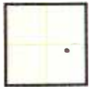
ONE POINT CAPTURE. SINGLE EVENT CAPTURE USING EQUIVALENT TIME SAMPLING. 20 MS/S, 100 MHz DSO.
