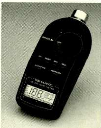
Radio Shack's Model 33-2055 digital SPL meter was used to measure the sound-pressure level at a middle-school dance.
