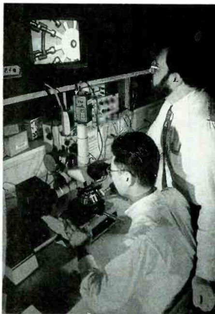
FIG. 1—MICROMACHINED microactuator made by integrated circuit fabrication techniques is examined under an electron microscope by Georgia Tech scientists, (left), and a microphotograph of a prototype planar, variable-reluctance magnetic micromotor (right).
