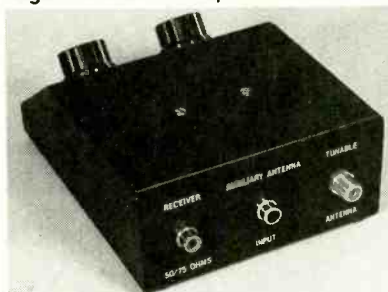
FIG. 4—ANTENNA CONTROLLER unit. House the controller in a metal case to provide RFI shielding.
