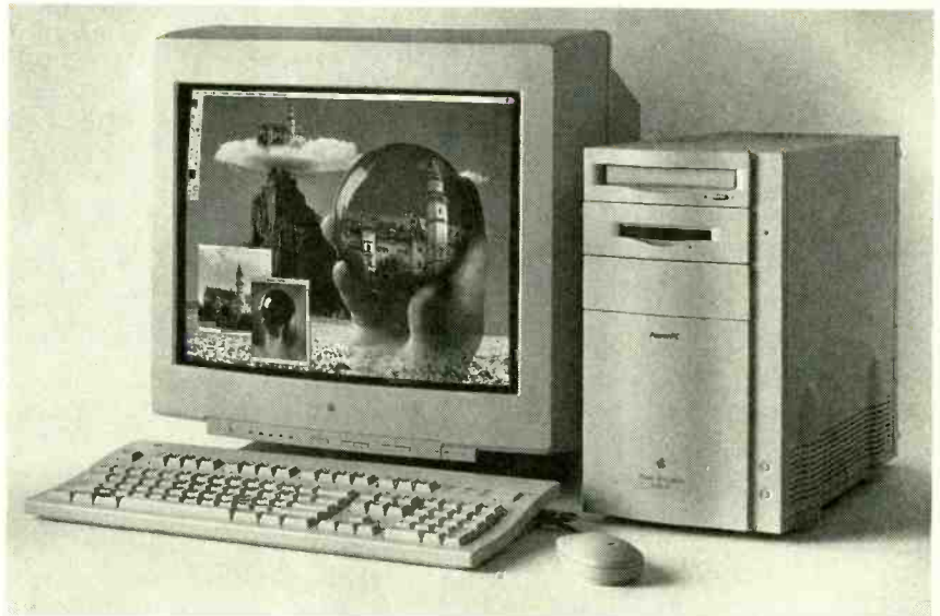
FIG. 1—APPLE'S NEW POWERPC-BASED MACINTOSH line introduces RISC-level performance at desktop prices. SoftWindows technology from Insignia Solutions lets DOS and Windows programs run in emulation mode at 486/25 speeds.
