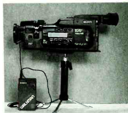
FIG. 11—THE FM RECEIVER CONNECTS to the external microphone input jack on your camcorder.
