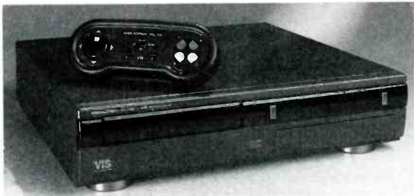
FIG.2—TANDY'S VIS or Video Information System runs a Windows-like operating system designed by Microsoft.
