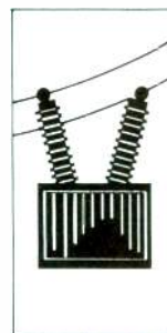
STEP-DOWN TRANSFORMER 5–20μT
