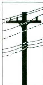
SECONDARY DISTRIBUTION LINES (115/230V) 0.1–1μT, WITH A SLOW MAGNETIC FIELD DROP-OFF OF 1/r (DUE TO UNBALANCED PHASE AND NEUTRAL LINES)
