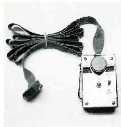
FIG. 7—THE HAND-HELD CONTROLLER allows you to “walk” the mower around the yard to cut a perimeter for it to follow.
