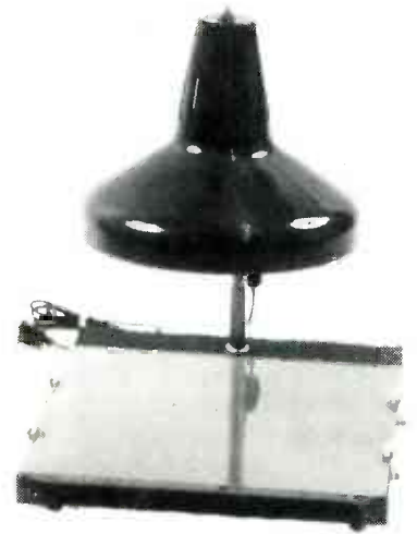
FIG. 3—TO EXPOSE THE BOARD, place the sensitized blank and the photomask in a contact frame and place under a strong light source.
