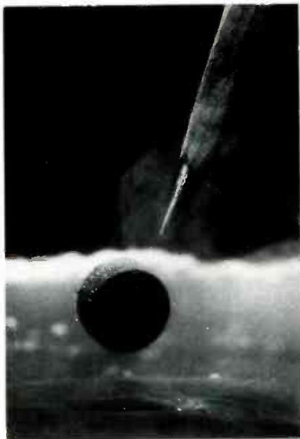
FIG. 1—A SUPERCONDUCTOR FLOATS IN air above a magnet. This experiment, which has come to symbolize the breakthroughs in superconductivity, demonstrates Meissner's effect, whereby magnetic flux does not enter a superconductive material. In effect, the superconductor looks like a "magnetic mirror."
