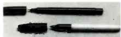
FIG. 7—PC ARTWORK CAN BE DRAWN directly on the copper blank using etch-resist pens. Lacquers and drafting aids can be used, too.
