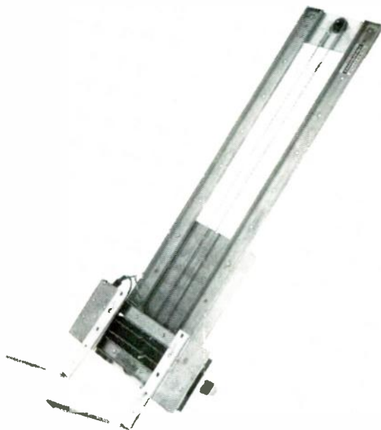
FIG. 1—THIS FORK-LIFT DESIGN can do almost as much as a multi-jointed arm, but with higher lifting capacity and at a lower cost. For greater dexterity, the pincher shown can be added. That pincher, part of which is shown here, will be described in detail in an upcoming installment of this series.
