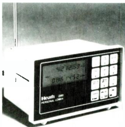
FIG. 6—By combining a computer with user-programmed memory, a relatively inexpensive Loran receiver such as this Heath Model 2980 Personal Loran can display location, bearing and time to waypoints, and even off-course direction.
