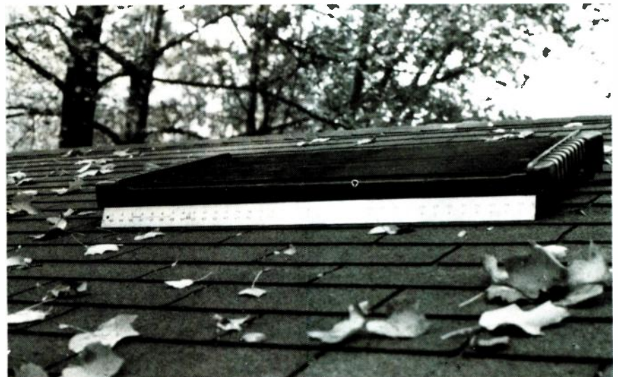
FIG. 1—THIS PROTOTYPE LIMPET GENERATOR, installed on a rooftop in Maryland, is but six inches high.
