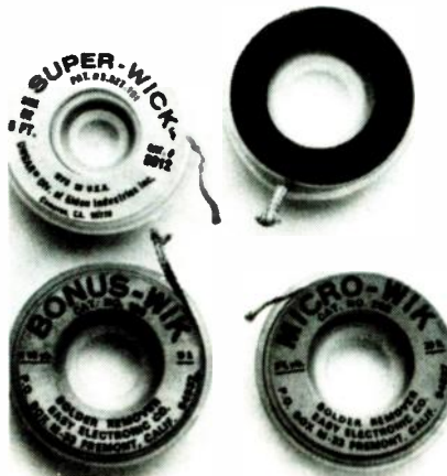
FIG. 6—SOLDER-REMOVAL BRAID is available in several widths to accommodate everything from hairline printed-circuit traces to old-fashioned terminal lugs.
