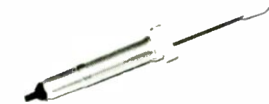
FIG. 7—A SOLDER-SUCKER removes solder from a one-surface component-mounting hole or a plated-through connection.
