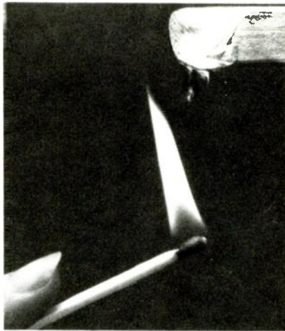
FIG. 9—THE HEAT FROM A MATCH is enough to melt a bar of indium fusible-alloy solder.
