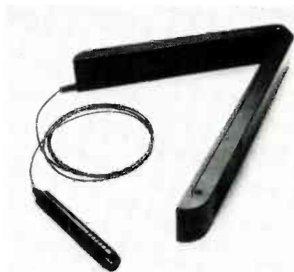
THE SPACE PEN from Soniture allows three-dimensional input to a computer.
