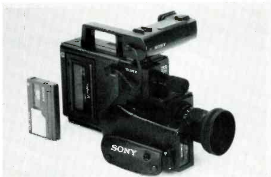
AN ALL-IN-ONE 8mm camcorder, the CCD-V8 from Sony can record two hours of video.
