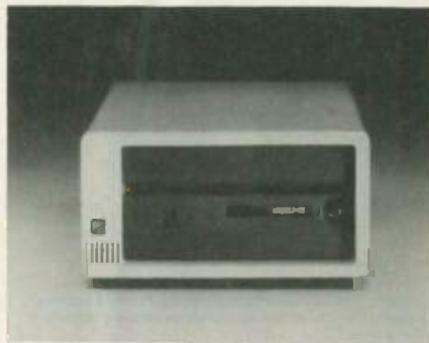
Fig. 1—THE RANA 2.5 SUPER FLOPPY-DISK SYSTEM is capable of storing 2.5 megabytes on a 5¼ inch floppy diskette. It, ushers in a new era in high-density storage devices.
