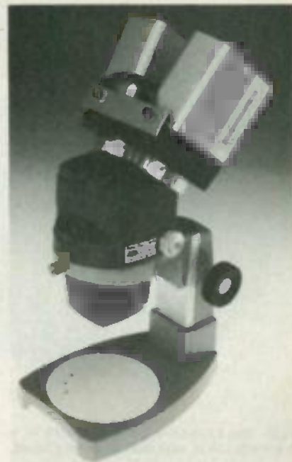
FIG. 3—ANOTHER 3-D IMAGE SOURCE. Here, twin video-cameras are mounted on a stereoscopic zoom-microscope to create a "3-D microscope."
