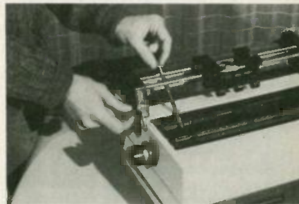
SLIDE THE SUPPLIED GAUGE —actually a notched rod—on the drive bar, tighten two screws, and the tractor assembly is adjusted for use.
