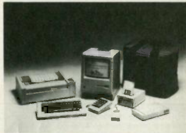
A VARIETY OF ACCESSORIES is available for the Macintosh, including an outboard drive, a numeric keypad, printer, modem, and carrying case.
