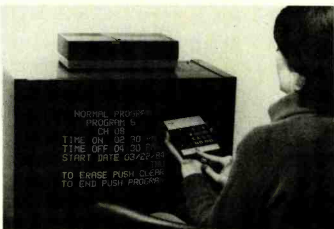
THE RCA VKP900 REMOTE-CONTROLLED VCR. The viewer is using her unit to review the programs stored in the memory. The alphanumeric display also assists the viewer in setting the equipment to record one-time daily, or weekly programs.
