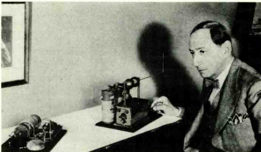
HUGO GERNSBACK at the key of the Telimco wireless transmitter. The receiver is at the left.
