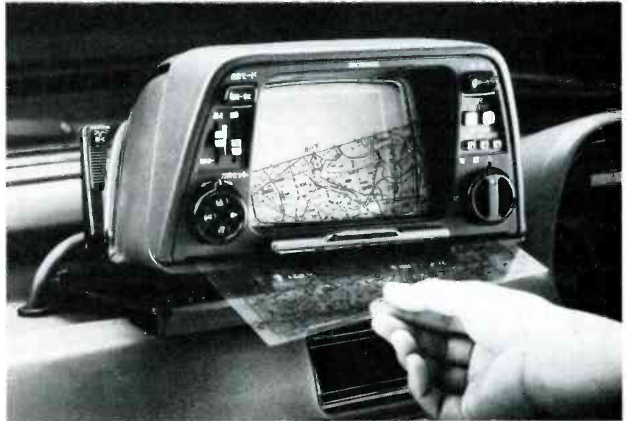
FIG. 4—IN THE ELECTRO GYRO-CATOR from Honda, the maps are on overlays that slip over a display that sits on top of the dashboard.
