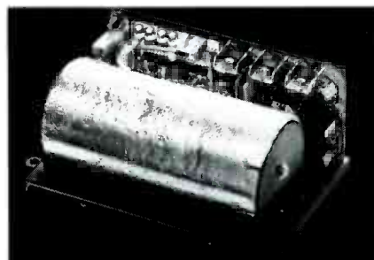
FIG. 5—THE DIRECTIONAL SENSOR contains a self-calibrating gyroscope. Its purpose is to advise the computer of any changes in direction.
