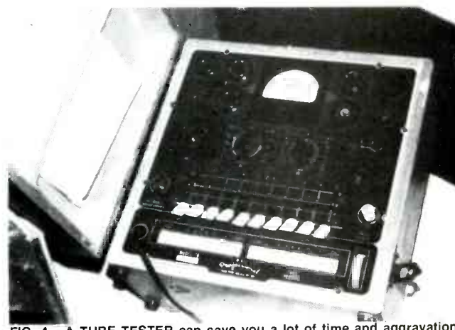
FIG. 4.—A TUBE TESTER can save you a lot of time and aggravation, especially if you buy a large numbers of used tubes.
