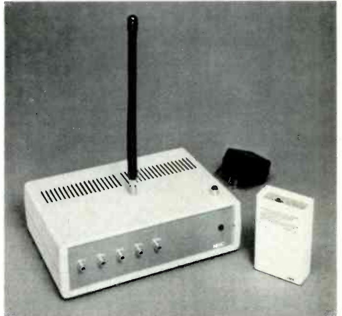
THE TACTILE COMMUNICATOR , with which the deaf or blind may receive signals they could not otherwise see or hear, at left; the pocket receiver at right.
