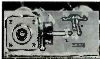
FIG. 18—DIODES D10-D13 are connected at one end to Teflon balun on top of mixer board. Wire loops L12 and L13 are described in text.
