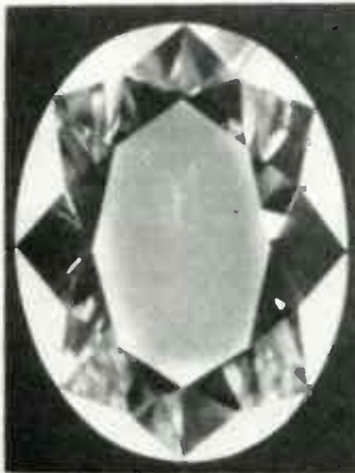
"BRANDED" DIAMONDS CAN be identified quickly and conveniently. The distinguishing mark (actually, an area of altered electrical conductivity) is normally invisible (left). To make it visible (right), the diamond is given an electrostatic charge and dusted with a special powder. That outlines the branded region—here, a heart-shaped pattern.
