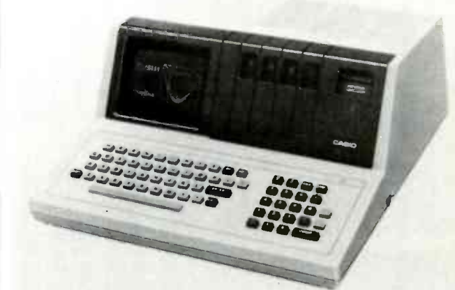
THE CASIO FX-9000P personal computer. The basic unit comes with a 4K RAM, a 5.5-inch built-in CRT, very extensive high-resolution graphics, and powerful mathematical functions for scientific, engineering and statistical operations.
