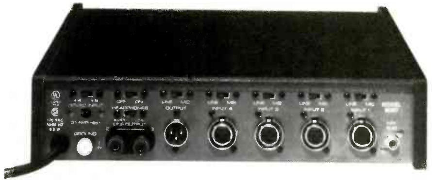
FIG. 1—A MIXER, such as the Shure M267, allows you to use several microphones or other audio sources.
