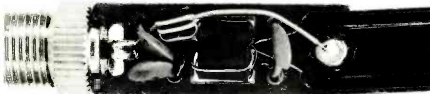
FIG. 13—BOARD FOUND INSIDE balun, showing addition of 10 \mu H choke and power leads.
