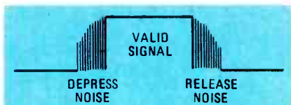
FIG. 12—KEY BOUNCE generates noise that can confuse the microprocessor when a key is pressed and released. The text explains how the valid signal is extracted.
